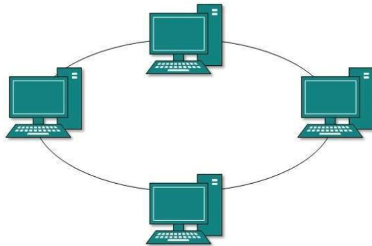
Ring topologies are resilient to cable failures but can suffer from performance degradation if a device fails or if the ring is interrupted.
