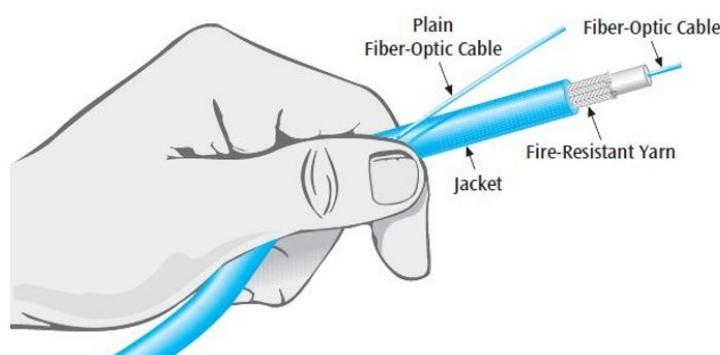
They offer high bandwidth, low attenuation, and immunity to electromagnetic interference. Fiber optic cables are widely used in long-distance telecommunications networks, backbone infrastructure, and high-speed Internet connections.
