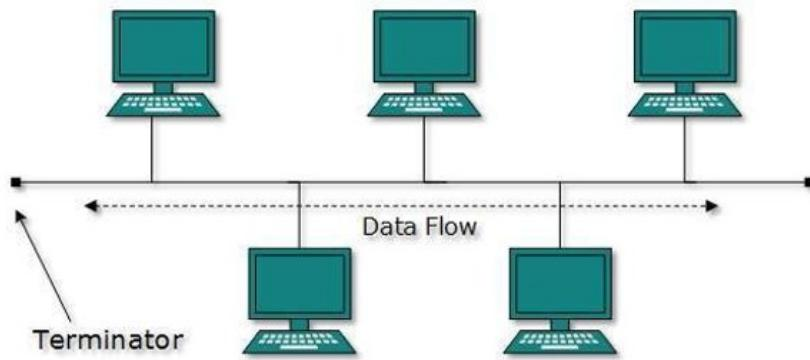
Bus topologies are simple and inexpensive but can suffer from signal degradation and limited scalability.
