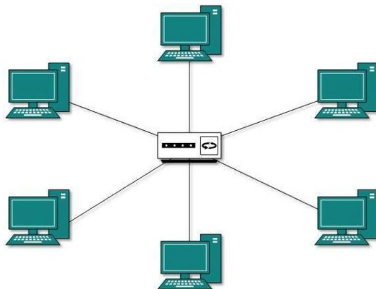
Data travels through the hub or switch, which manages communication between devices.
